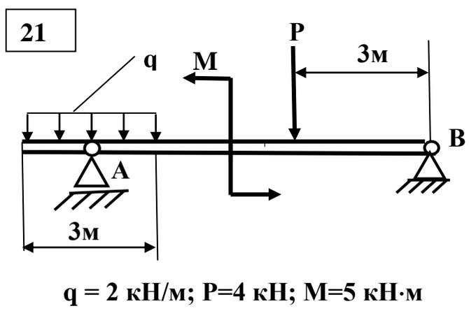
$q = 2 \text{ кН/м}; P = 4 \text{ кН}; M = 5 \text{ кН м}$
