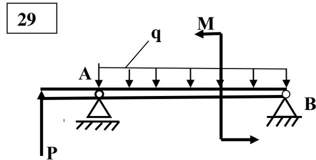
$$q = 1 \text{ кН/м}; P=3\text{кН}; M=4 \text{ кН}\cdot\text{м}$$
