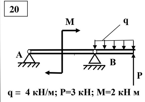
$q = 4 \text{ кН/м}; P = 3 \text{ кН}; M = 2 \text{ кН м}$
