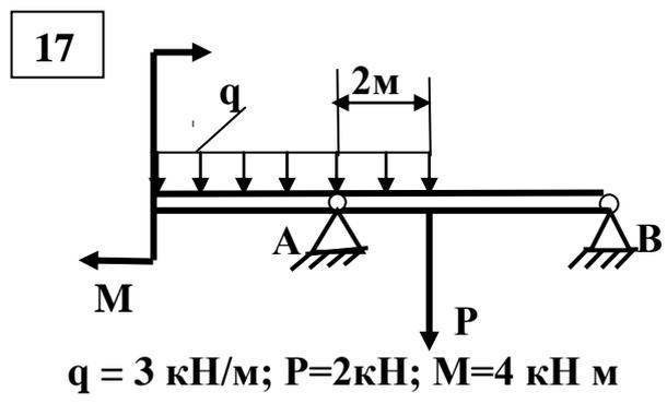
$q = 3 \text{ кН/м}; P = 2 \text{ кН}; M = 4 \text{ кН м}$
