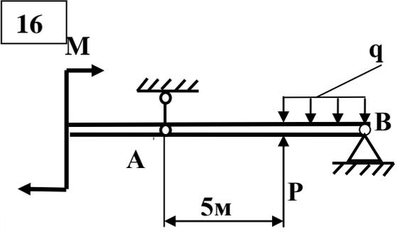
$P = 3 \text{ кН}; q = 2 \text{ кН/м}; M = 2 \text{ кН м}$
