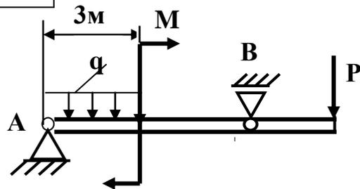
$q = 2 \text{ кН/м}; P = 4\text{кН}; M = 3 \text{ кН м}$
