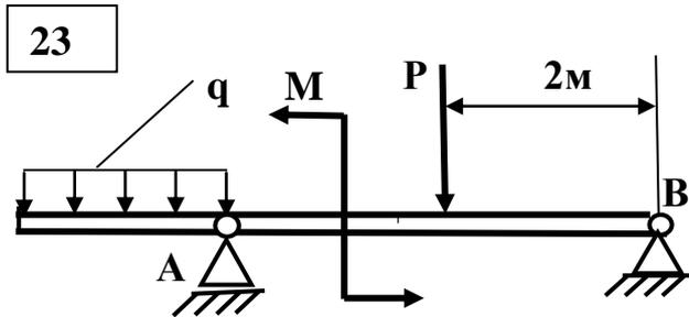
$$q = 3 \text{ кН/м}; P=5 \text{ кН}; M=4 \text{ кН}\cdot\text{м}$$
