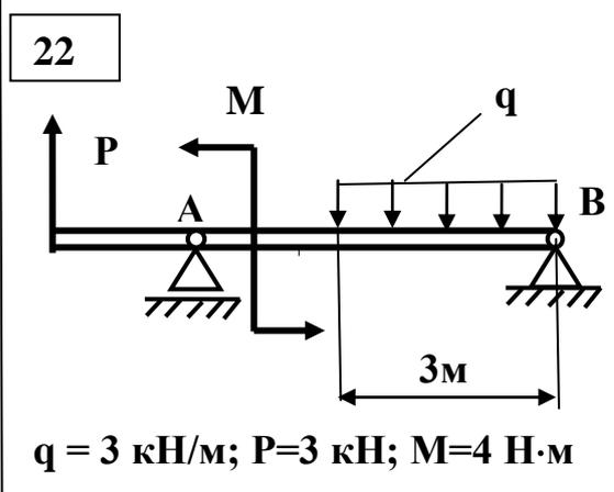
$q = 3 \text{ кН/м}; P = 3 \text{ кН}; M = 4 \text{ кН м}$
