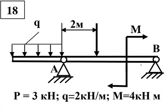
$P = 3 \text{ кН}; q = 2 \text{ кН/м}; M = 4 \text{ кН м}$
