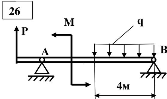
$$q = 3 \text{ кН/м}; P=2 \text{ кН}; M=6 \text{ кН}\cdot\text{м}$$
